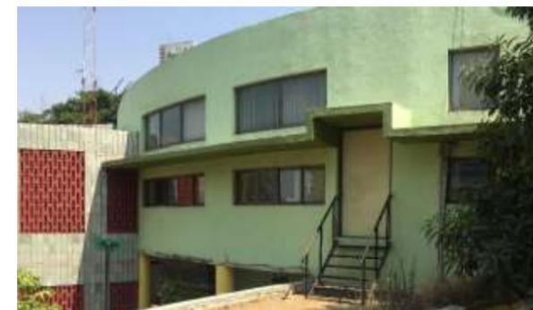
▲ Design of façade in two levels – ‘top’ and ‘bottom’ window help in receiving optimum daylight. Top window acts as a light shelf and bottom window serves the purpose of visual connectivity
