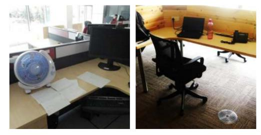
Controllability is an important aspect of individual thermal comfort. Provide desk fans and under floor air distribution system to enable occupants in maintaining air movement based on their preference
